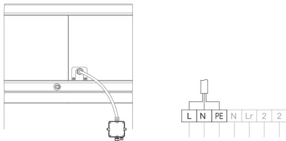
Figure 9b: Installing a power cord
