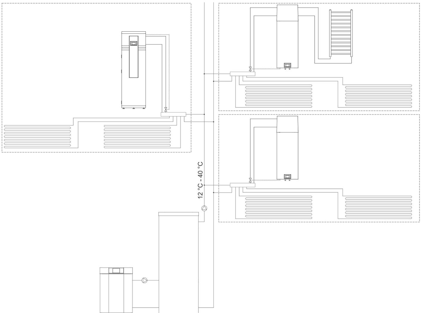
Fig. 3: Possible installation of a heat pump
