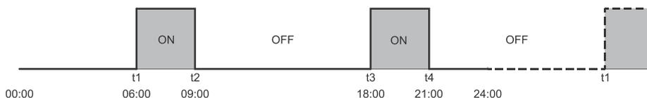
Figure 13: Example of setting the timer – radiator heating
