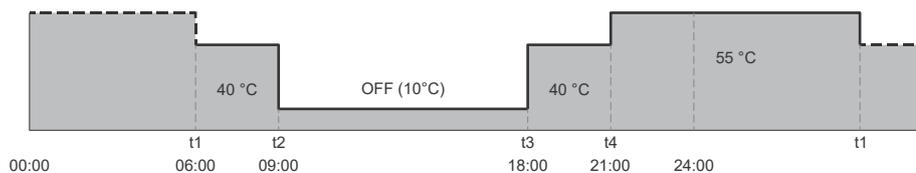
Fig. 12: Example of setting the timer
