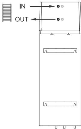
Inlet and outlet of pipes for connecting to a radiator are on the back side of the heat pump marked with IN and OUT. The return pipe is marked with IN, and the flow pipe with OUT. The heat pump can be connected to a radiator with a max power of 700 W as per EN 442 (inlet temp. 65 °C), which is around 300 W at the operating inlet. Maximum distance between the radiator and the heat pump is 8 m.
